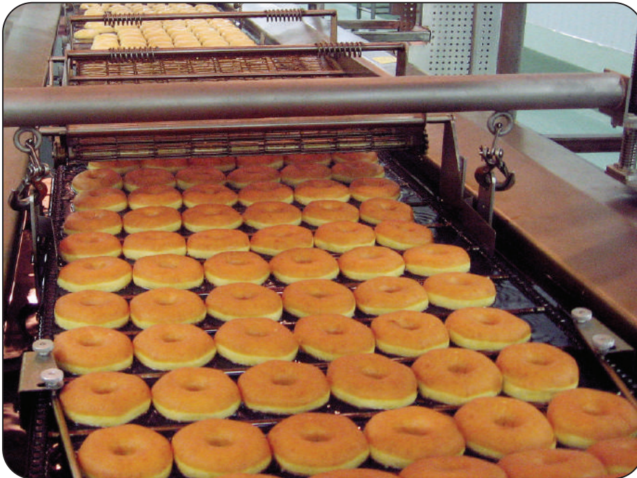
Century 6-16E Donut Line Capacity 137 dozen/hour @100 seconds frying time
