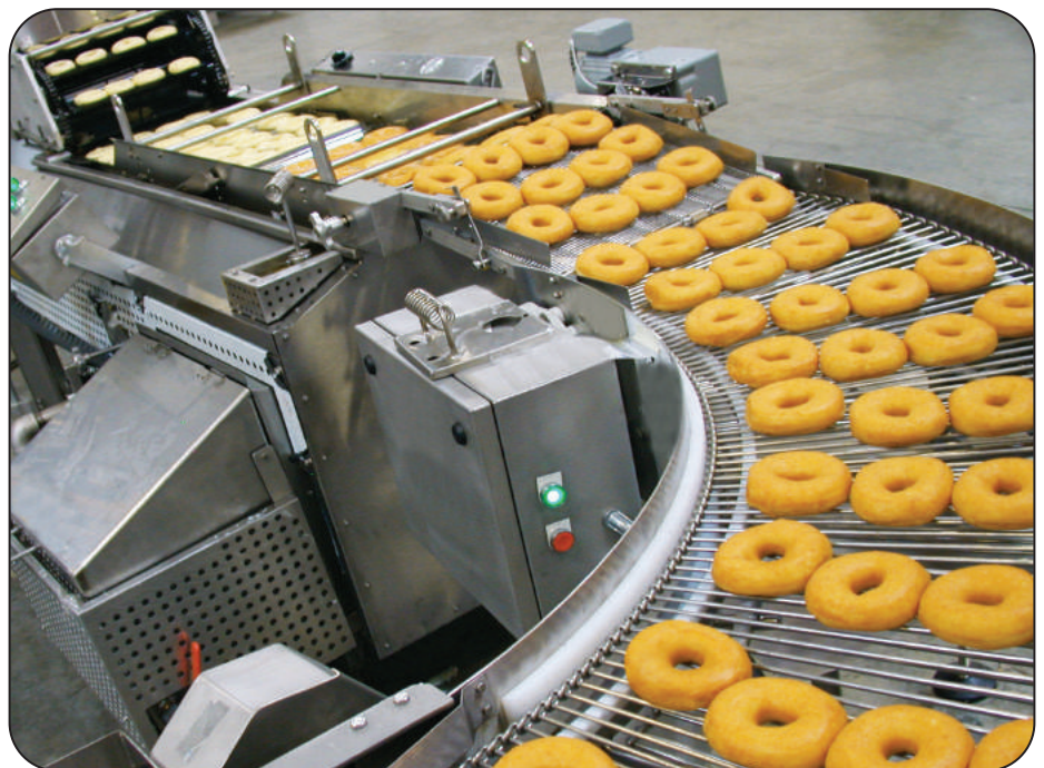
Century 16-36G Donut Line Capacity 930 dozen/hour @100 seconds frying time
